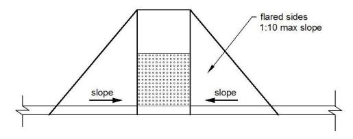
Figure 11B-406.2.2 Sides of Curb Ramps
