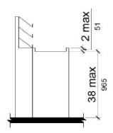
Figure 11B-904.3.2 Check-Out Aisle Counters
