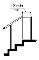
Figure *11B*-505.10.2 Top Handrail Extension at Stairs
