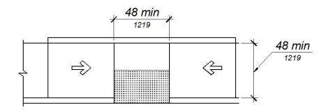
Figure 11B-406.3.2 Parallel Curb Ramps
