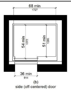
Figure 11B-407.4.1 Elevator Car Dimensions
