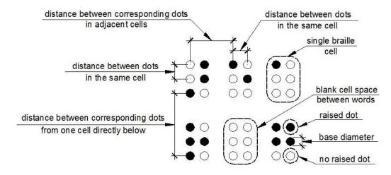
Figure 11B-703.3.1 Braille Measurement
