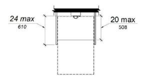
Figure 11B-704.2.1.2 Forward Approach to Telephone
