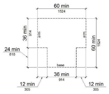
Figure 11B-304.3.2 T-Shaped Turning Space
