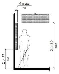
Figure 11B-307.2 Limits of Protruding Objects
