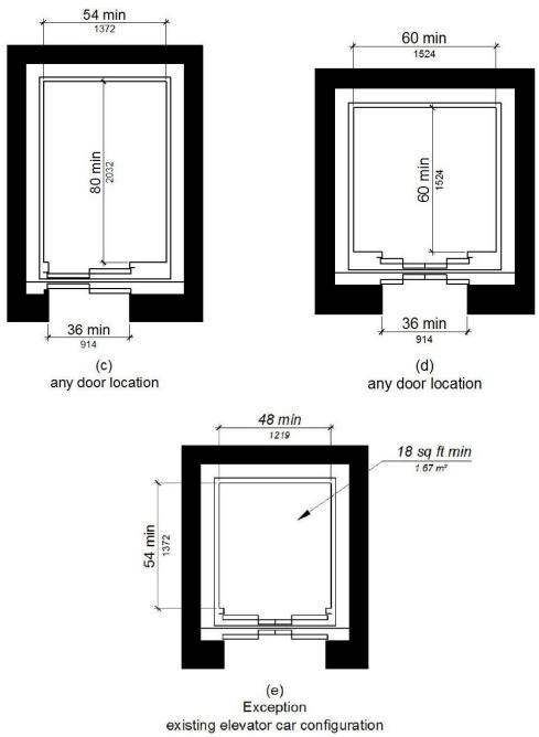
Figure *11B-*407.4.1 Elevator Car Dimensions
