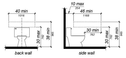
FIGURE 11B-809.10.7.3 REINFORCEMENT FOR GRAB BARS.
