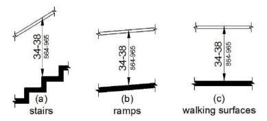
Figure 11B-505.4 Handrail Height
