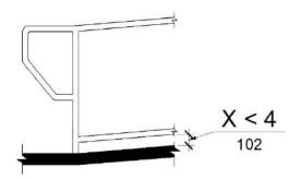
Figure 11B-405.9.2 Curb or Barrier Edge Protection
